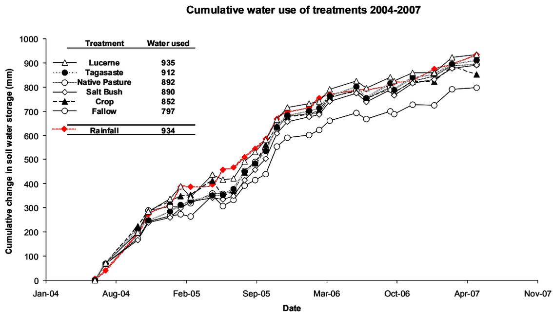
Figure 1. Cumulative monthly rainfall (mm) and the cumulative change in soil-water storage (mm) between depths 0-180cm, under the 6 treatments from 2004-2007 at Boolite.
