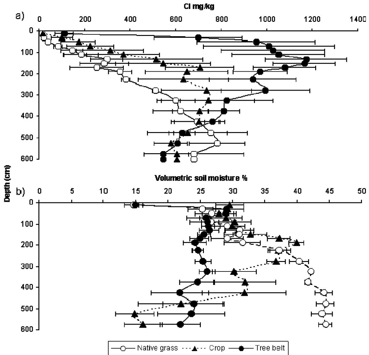
Figure 2. Distribution of chloride (Figure 2a) and water (Figure 2b) down the soil profile at Boolite under three different landuses to 600 cm.
