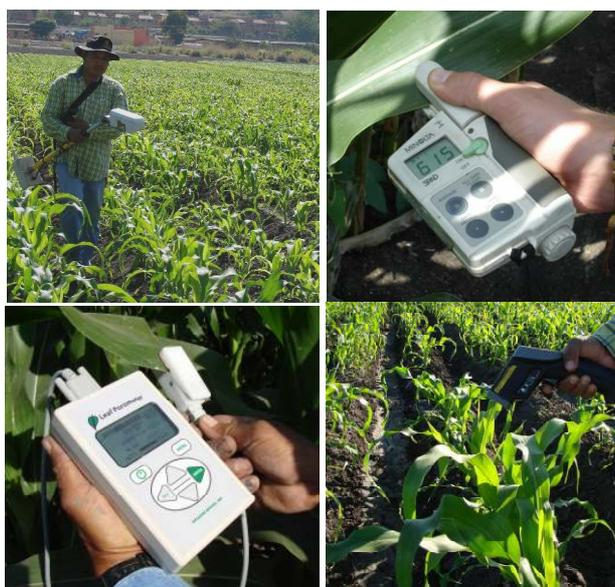
**Figure 1.** Different devices used in this study to evaluate plant growth, phenology and water status: Spectroradiometer with active sensor to measure NDVI (upper left), leaf chlorophyll meter (upper right), porometer to measure stomatal conductance (lower left) and infrared thermometer to measure leaf temperature (lower right).
