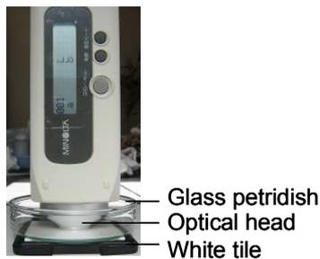
**Figure 1. Calibration of Minolta Colour Reader (CR-13).**
