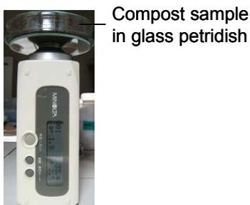
**Figure 2. Measurement of compost color using Minolta Colour Reader (CR-13).**
